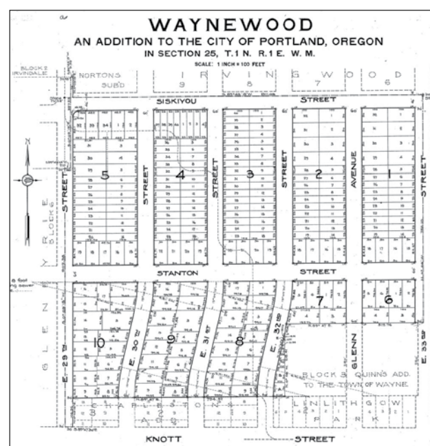
THE OFFICIAL PLAT OF WAYNEWOOD FILED WITH THE MULTNOMAH COUNTY SURVEYOR ON FEBRUARY 2, 1918 CONTAINING THE BRAND-NEW RETITLED LOTS AND REDRAWN STREETS. IN ADDITION TO UNDERSTANDING HOW THE CURVES CAME TO BE, THE REPLATTING PROCESS ALSO EXPLAINS THE MISALIGNED CORNER AT NE 29TH AND SISKIYOU.
